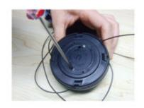
the battery box with Open screwdriver, then place a battery into
