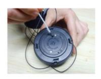
When keep pressing the reset button, the buzzer will alarm continuously and the red LED will flash continuously; When release the reset button, the buzzer will stop alarming and the red LED will flash every 6 seconds. When the AS1008 is alarming, press the reset button, and the alarming will stop and when release the reset button the AS1008 will be back to the normal working status.
