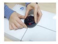
Place the item on the bottom plate, press the lock plunger, then rotate the top plate clockwise, until it is locked tightly.
