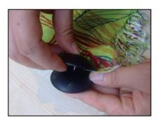
Insert the lock bulb into detacher, move the pin and separate the tag from the merchandise.
