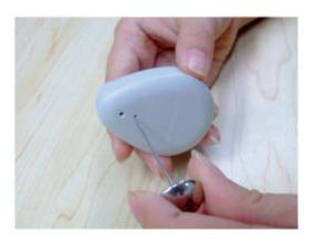
Keep pressing the reset button, the buzzer will alarm continously, and the LED will flash continously, until the pressing on the Reset Key is released; Meanwhile, applying a click on the reset button, the selfalarm of the tag will be turned off.
